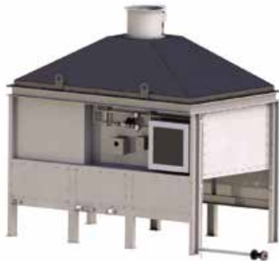
FLAME OFF STATION For alcohol based coating
