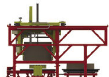
Step 4 - Cope half is centred on the 'y' axis, lifted and rotated through 180 degrees
