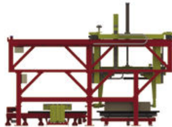
Step 2 - Drag half is centred on the 'y' axis, lifted and placed onto the casting pallet
