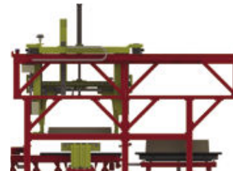
Step 3 - Cope half is centred on the 'x' axis
