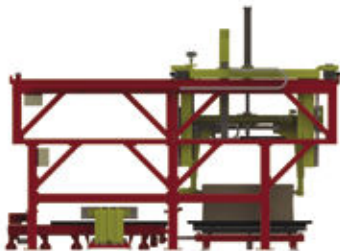
Step 5 - Cope half is closed onto the Drag half. Precise alignment ensured by use of a floating table
