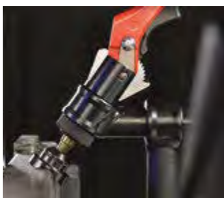
Pressure and support pieces with V-block Clamping of round/rectangular tubes
